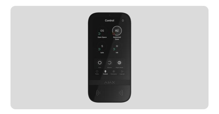
**KeyPad TouchScreen** is a wireless keypad with touch screen for Ajax security system management. Users can authenticate using smartphones, <u>Tag</u> key fobs, **Pass** cards and codes. The device is designed for indoor use.
