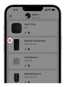
When a KeyPad TouchScreen malfunction is detected, the Ajax app displays a malfunction counter on the device icon. All malfunctions are shown in the keypad states. Fields with malfunctions will be highlighted in red.
