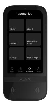
The separate keypad tab holds up to 6 buttons which control one <u>automation</u> <u>device</u> or a group of devices. Group scenarios provide more convenient control of several switches, relays, or sockets simultaneously.
