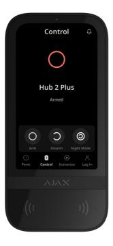
KeyPad TouchScreen can arm and disarm the entire object or separate groups, and activate **Night mode**. Use the **Control** • tab to change the security mode. You can control the security with KeyPad TouchScreen using:
