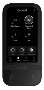
KeyPad TouchScreen allows to control the groups' security (if **Group mode is enabled**). You can also adjust in the keypad **settings** which groups will be shared (keypad groups). By default, all groups are available for viewing on the keypad display in the **Control** • tab. You can learn more about group security management in **this section**.
